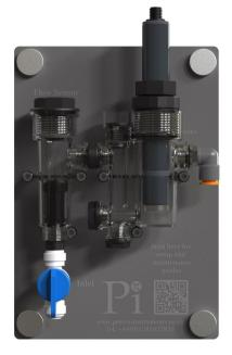
Designed specifically with online measurement in mind, these electrode-based sensors use a specialised electrolyte held within a membrane cap; this membrane allows  $CIO_2$  to diffuse into the electrolyte, where the following takes place at the electrodes:
